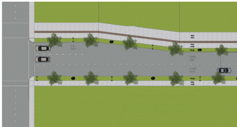
Figure 4.10: Plan view of Parkway Street showing flare outs at intersection
