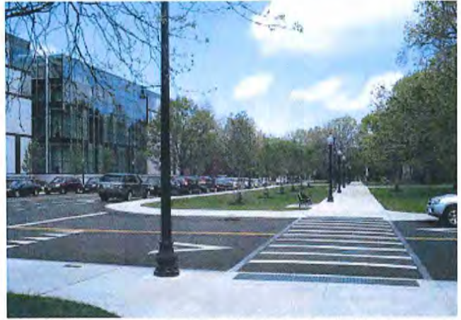
Figure 3.26 Example of a pedestrian-friendly crosswalk. Photo credit: NACTO.
