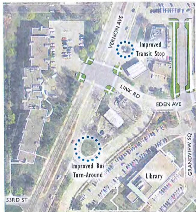
Figure 3.47 Diagram of proposed improvements to the transit system in the Short Term; 1" = 200'.
