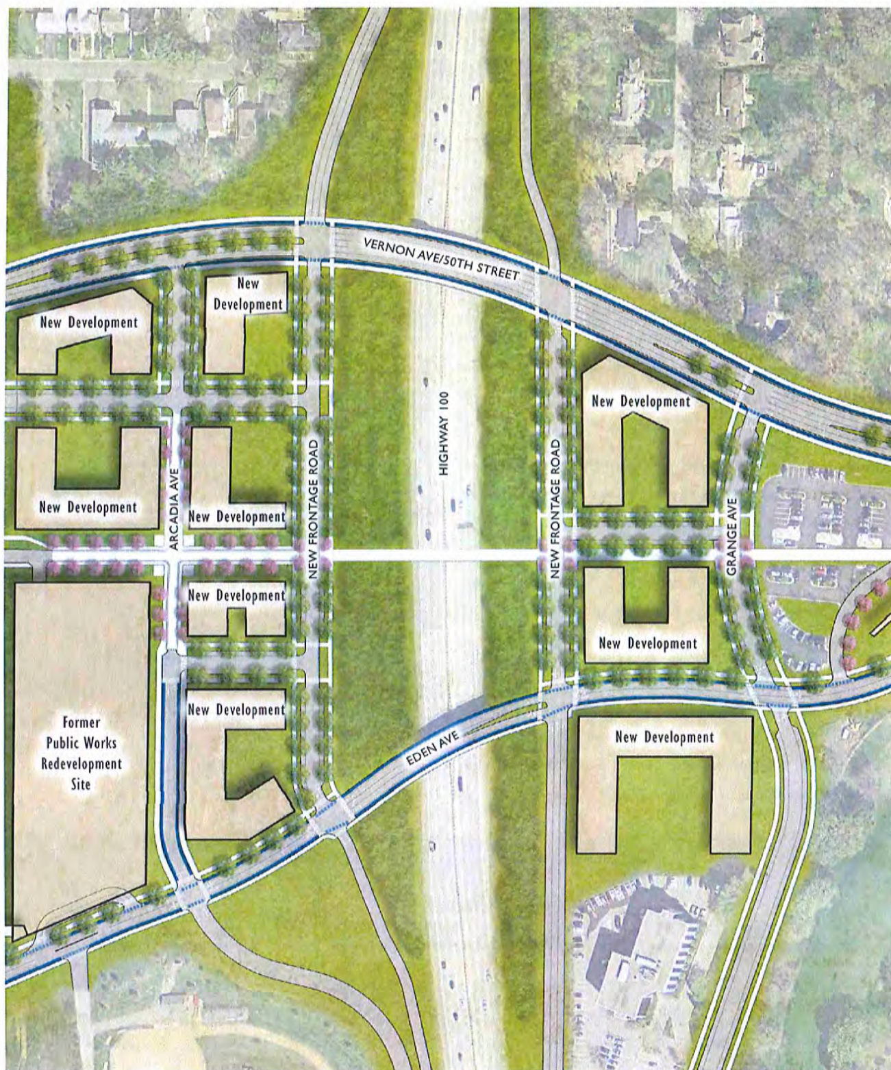
Figure 3.39 Plan of the new ramp configuration on the west and east sides of Highway 100, showing the integration of the ramp system with the District road network, servicing new developable parcels; 1" = 200'.
