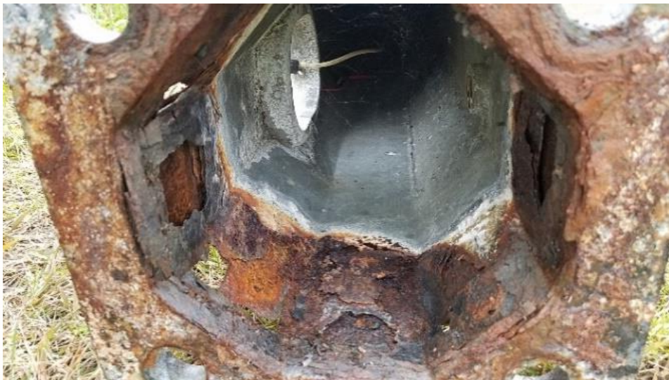
Photo 2. Internal Rusting of Streetlight Pole
