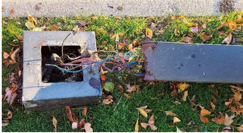
Photo 1. Failure Due to Rusting Streetlight Pole
