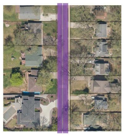
Can fit roughly two 15-ft wide storage vaults in the street width (or in the right-of-way).
