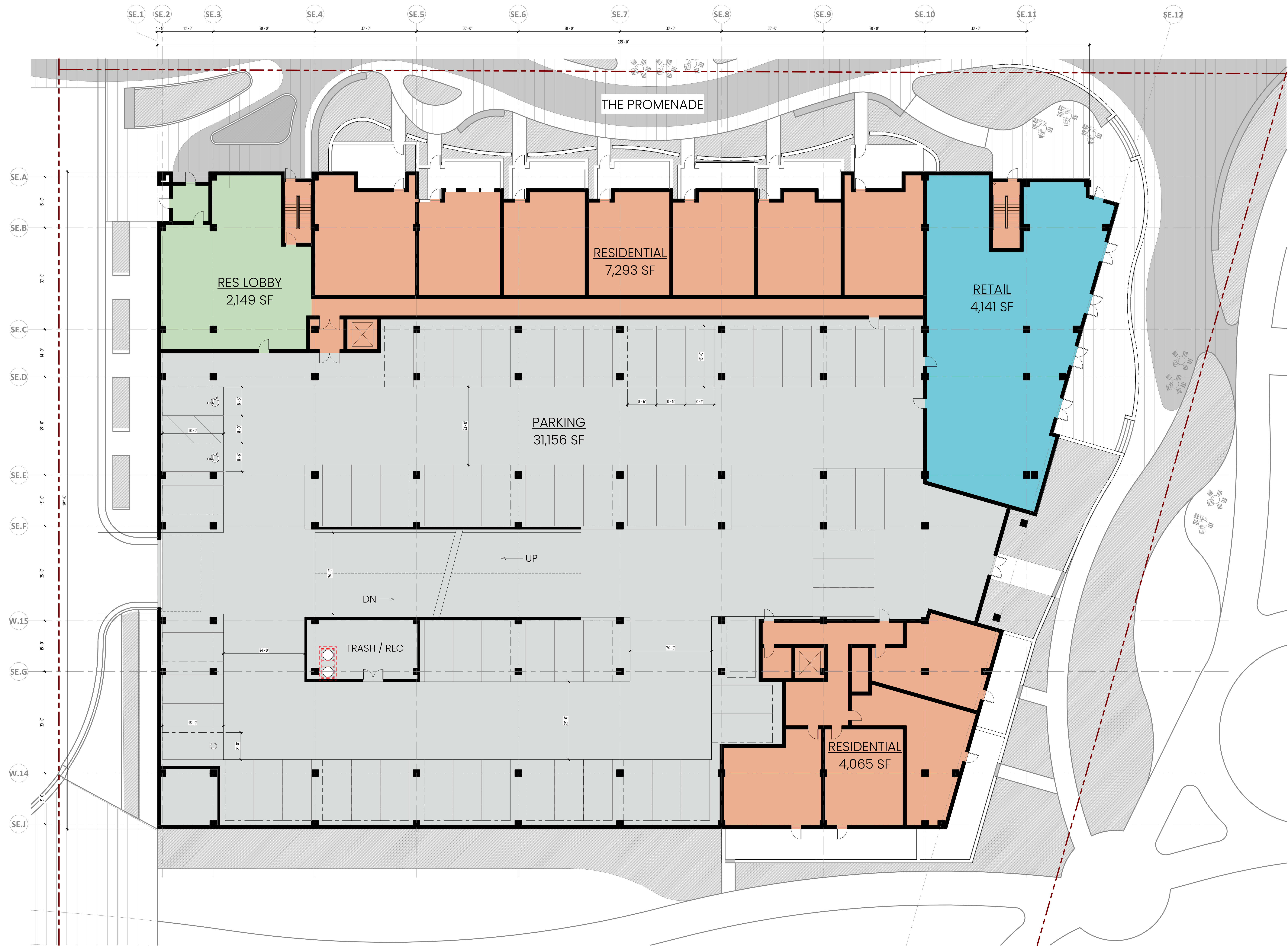
1 LEVEL 1 FLOOR PLAN - SOUTHEAST BUILDING A102-SE 3/32" = 1'-0"
